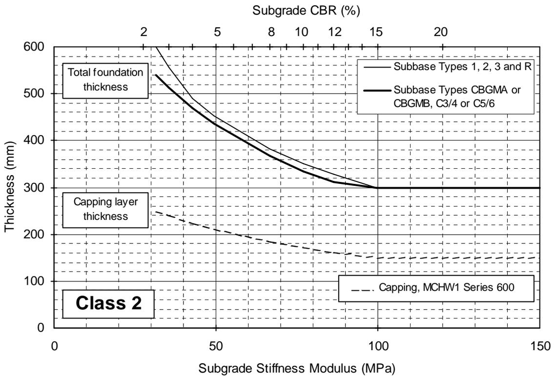
**FIGURE 4.2 Restricted Design Options – Class 2 Subbase on Capping**
