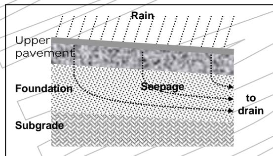
**FIGURE 6.1 Foundation Drainage**
