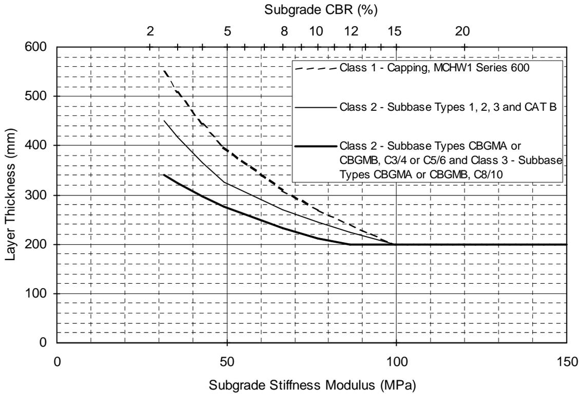
**FIGURE 4.1 Restricted Design Options – Subbase or Capping only**
