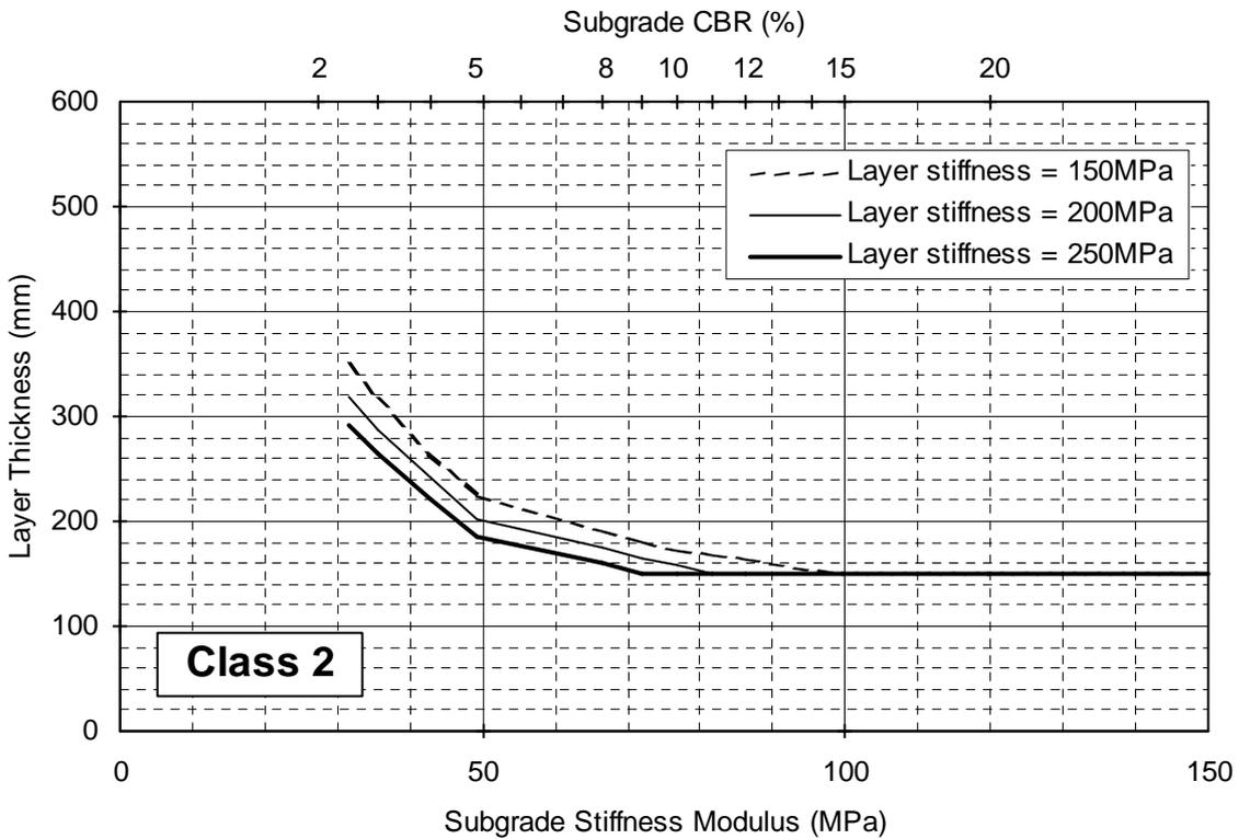
**FIGURE 5.3 Class 2 Designs – Single Foundation Layer**
