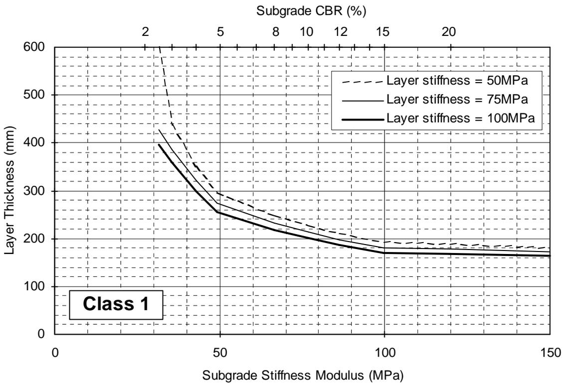
**FIGURE 5.2 Class 1 Designs – Single Foundation Layer**
