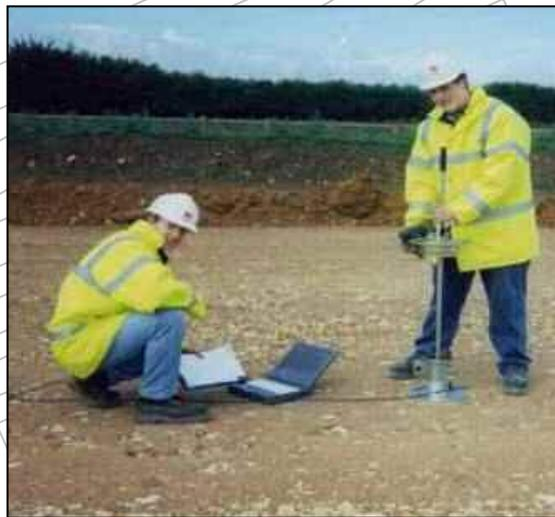
**FIGURE B.1 Dynamic plate Test**
