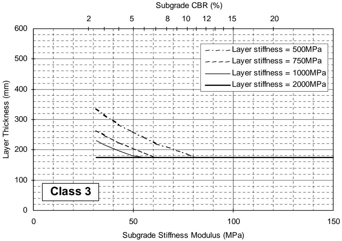
**FIGURE 5.4 Class 3 Designs – Single Foundation Layer**
