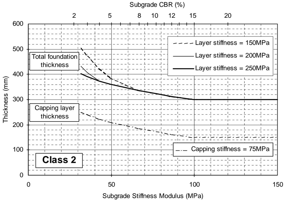
**FIGURE 5.6 Class 2 Designs – Subbase on Capping**
