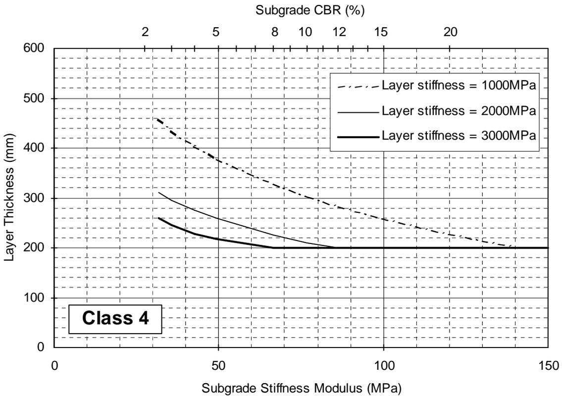
**FIGURE 5.5 Class 4 Designs – Single Foundation Layer**
