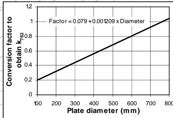
**FIGURE 7.3 Conversion Factors for Smaller Plate Sizes**
