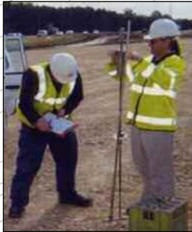
**FIGURE A.1 The Dynamic Cone Penetrometer**
